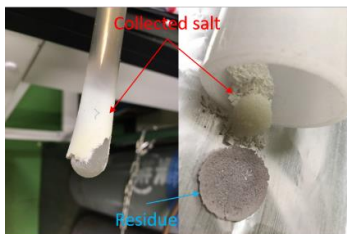
Fig.1 Collected salt and residue (vertical structure)
