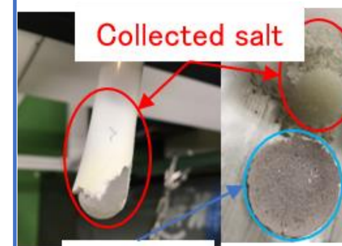
Collected salt and residue (NaCl-2CsCl 200V)
